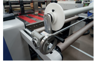
Adjustable feeding depending on material sizes and thickness. Vertical cardboard input control for efficient and fast feeding.
